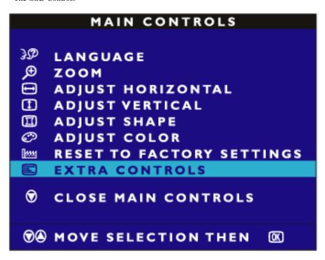
3) Press the button. The EXTRA CONTROLS window appears. ADJUST MOIRE will be highlighted.
